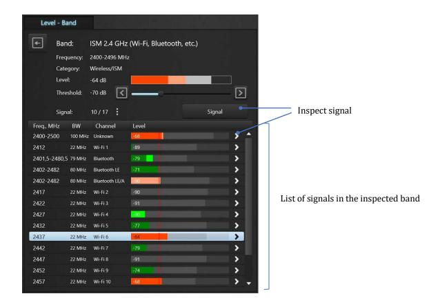
In this mode, only the selected band is scanned, its parameters and the list of signals within the band are displayed. For each of the signals, the frequency, band, channel name, current, peak, and maximum registered level are displayed.
