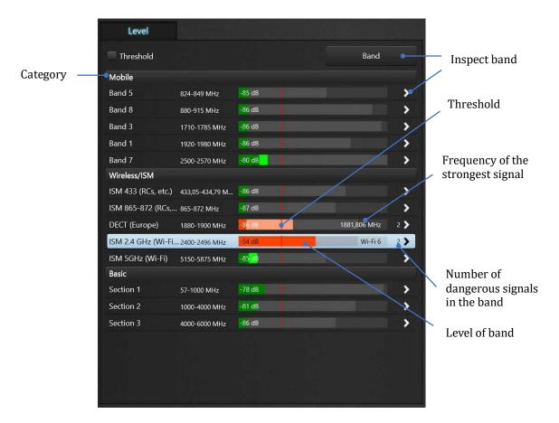
The operator can inspect the dangerous band by pressing the **Band** button or the arrow near the band. When the Level panel is in the band inspection mode, it displays the level of the selected band and a list of signals in the band. A bargraph is displayed for each of the signals. It changes color when the threshold is exceeded. The user can select a dangerous signal and proceed to its inspection.
