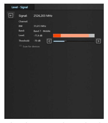
In this mode a separate signal is scanned. Use the signal inspection mode to study and locate the transmitter if it has a fixed frequency.
