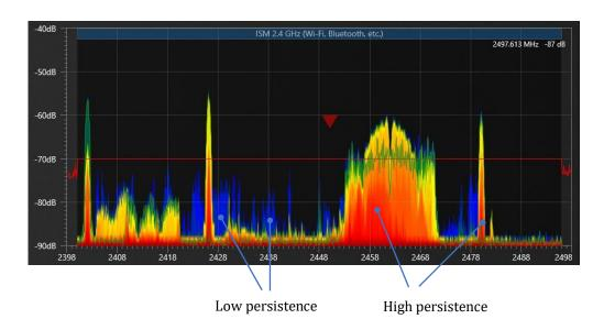
**Max level.** Sets the upper limit of the vertical scale of the spectrum graph. Choose a higher value to display stronger signals, and a lower value for better visual identification of weaker signals. Valid values are from -70 dB to -20 dB or "Auto". When using "Auto", the spectrum graph will adjust its vertical scale automatically.
