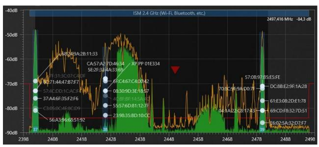
The device's level will change when the system is moved. Comparing the change in the spectral level with the change in the position of the blue icon can provide additional information about the signal. Simultaneous increase of both values will indicate that you are approaching the access point. If only the spectral level increases, and the level of the blue icon decreases or remains unchanged, you might be approaching a device that is a client of a distant access point.
