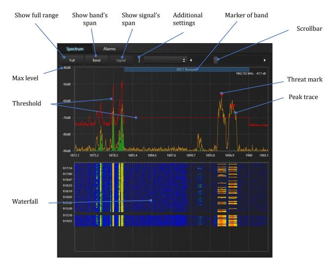
On the spectrum graph, the user can view any area, for example, the entire frequency range covered by the device, a band or a separate signal.
