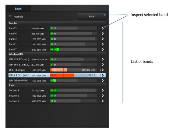
All bands according to the selected mode are scanned and displayed on the panel. The name, description, frequency, level (current, peak, and maximum recorded), as well as the number of dangerous signals and the most dangerous signal are displayed for each band. Bands are grouped by category.
