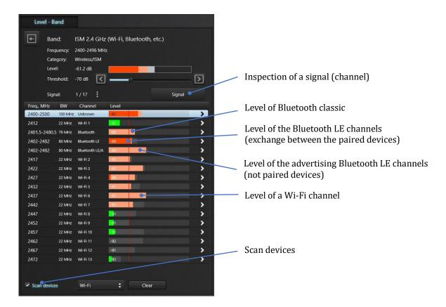
The Wi-Fi access points and not paired BLE devices can be scanned with the help of the computer's hardware and can be displayed on the spectrum graph and in the list.
