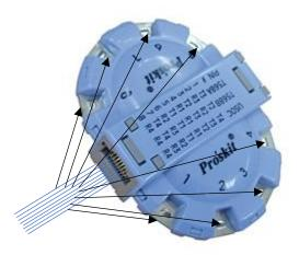
Since it is often unclear what particular conductors are used, all the combinations of the alligators can be used for checking the line: 1 and 2, 2 and 3, 3 and 4, 1 and 3, 1 and 4, etc. The spectrum may coinside in some pairs.
