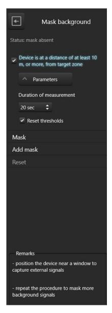
Enter the "Mask background" menu and confirm the correct placement by setting the checkbox "Device is at a distance of least 10 m, or more, from target zone". Then click "Mask" and wait for the result.
