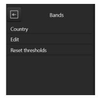
For the successful operation of the system, it is very important that the table of bands corresponds to the allocation of mobile and wireless bands that exist in the place of use. Fortunately, the "Breeze RF" software includes a data file that carries information about the frequency allocation in many countries and regions.
