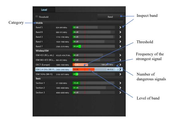
The operator can inspect the dangerous band by pressing the **Band** button or the arrow near the band. When the Level panel is in the band inspection mode, it displays the level of the selected band and a list of signals in the band. A bargraph is displayed for each of the signals. It changes color when the threshold is exceeded. The user can select a dangerous signal and proceed to its inspection.
