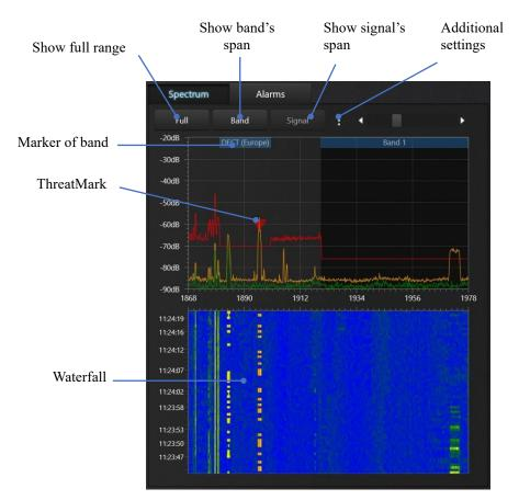
On the spectrum graph, the user can view any area, for example, the entire frequency range covered by the device, a band or a separate signal. Signal levels from -90 to -20 dB are displayed. The spectrum graph will automatically adjust its vertical scale to the maximum level being displayed.
