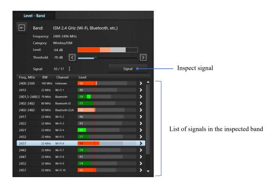
In this mode, only the selected band is scanned, its parameters and the list of signals within the band are displayed. For each of the signals, the frequency, band, channel name, current, peak, and maximum registered level are displayed.
